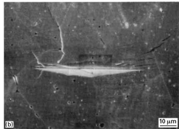
Figure 5 Microstructures of Knoop indentations as a function of load on polycrystalline \text{BaTiO}_3 : (a) 0.25 N; (b) 2 N.
